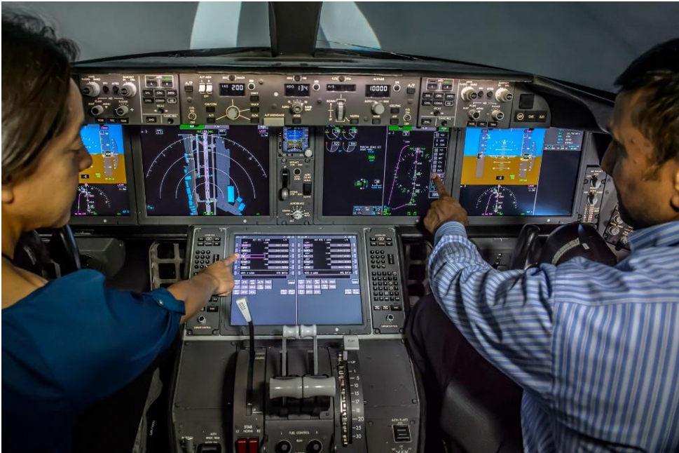
Figure 2: Large TSDs used in deck of the Boeing 777-x [21]
