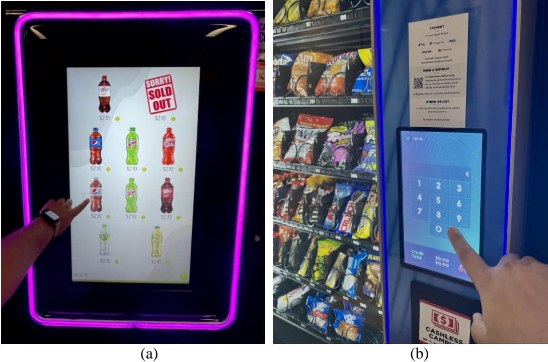
Figure 1: (a) TSD-based kiosk for point-of-sale purposes (b) Vending machine using large TSD for user input.
